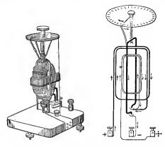
FIG. 161. View and diagram of the Siemen's electro-dynamometer.
